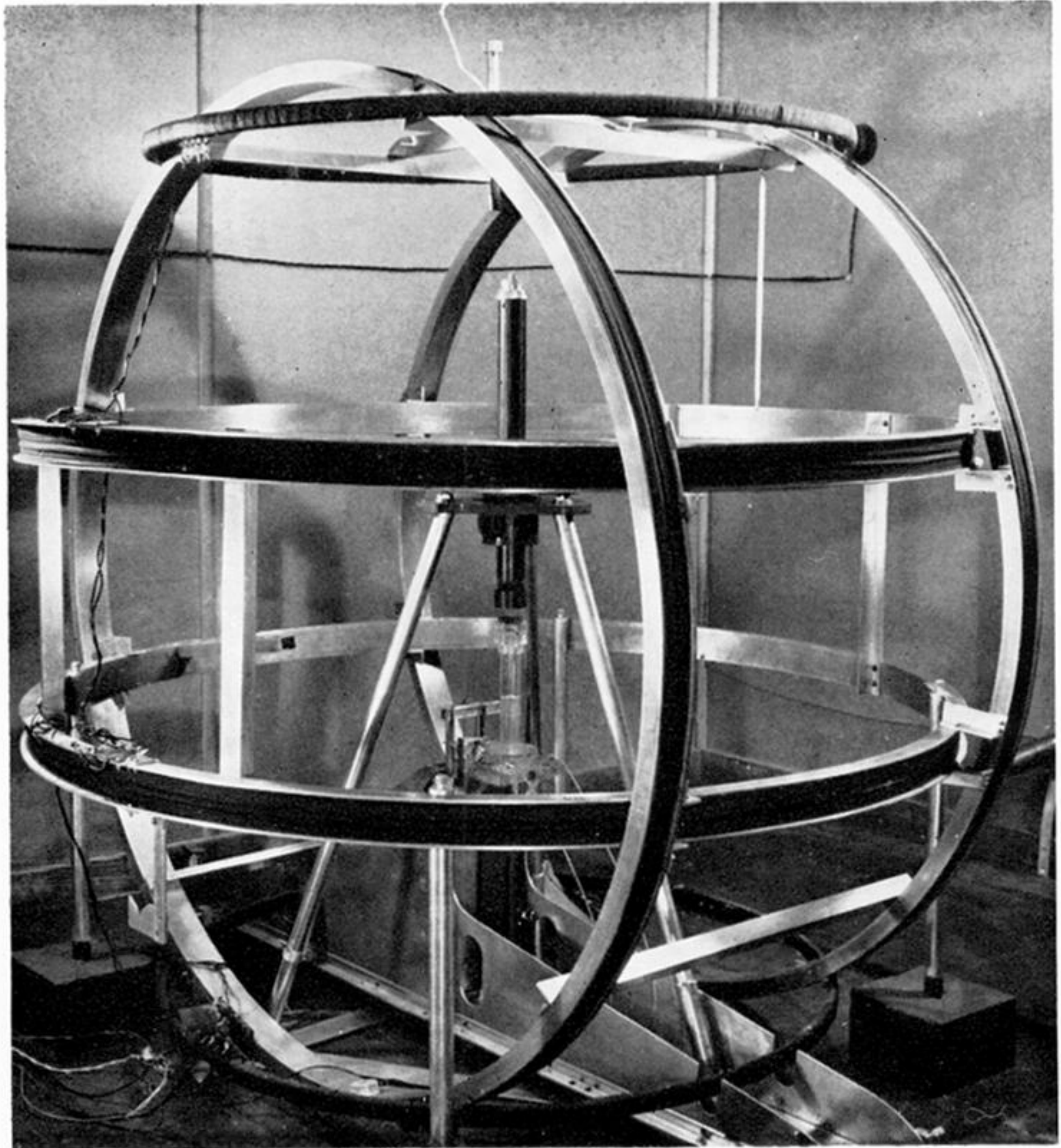
FIGURE 3. Magnetometer with Fanselau and Helmholtz coil systems.
