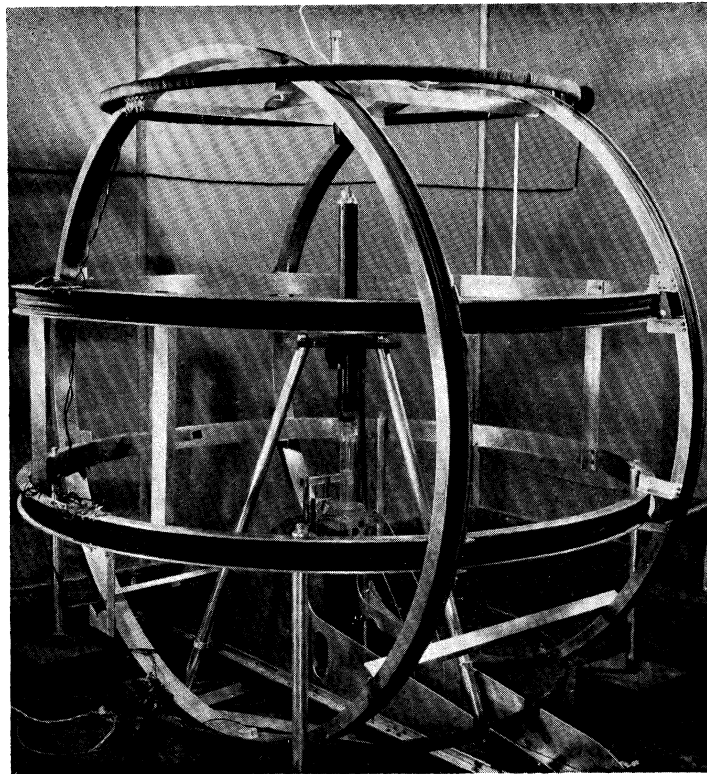
FIGURE 3. Magnetometer with Fanselau and Helmholtz coil systems.
